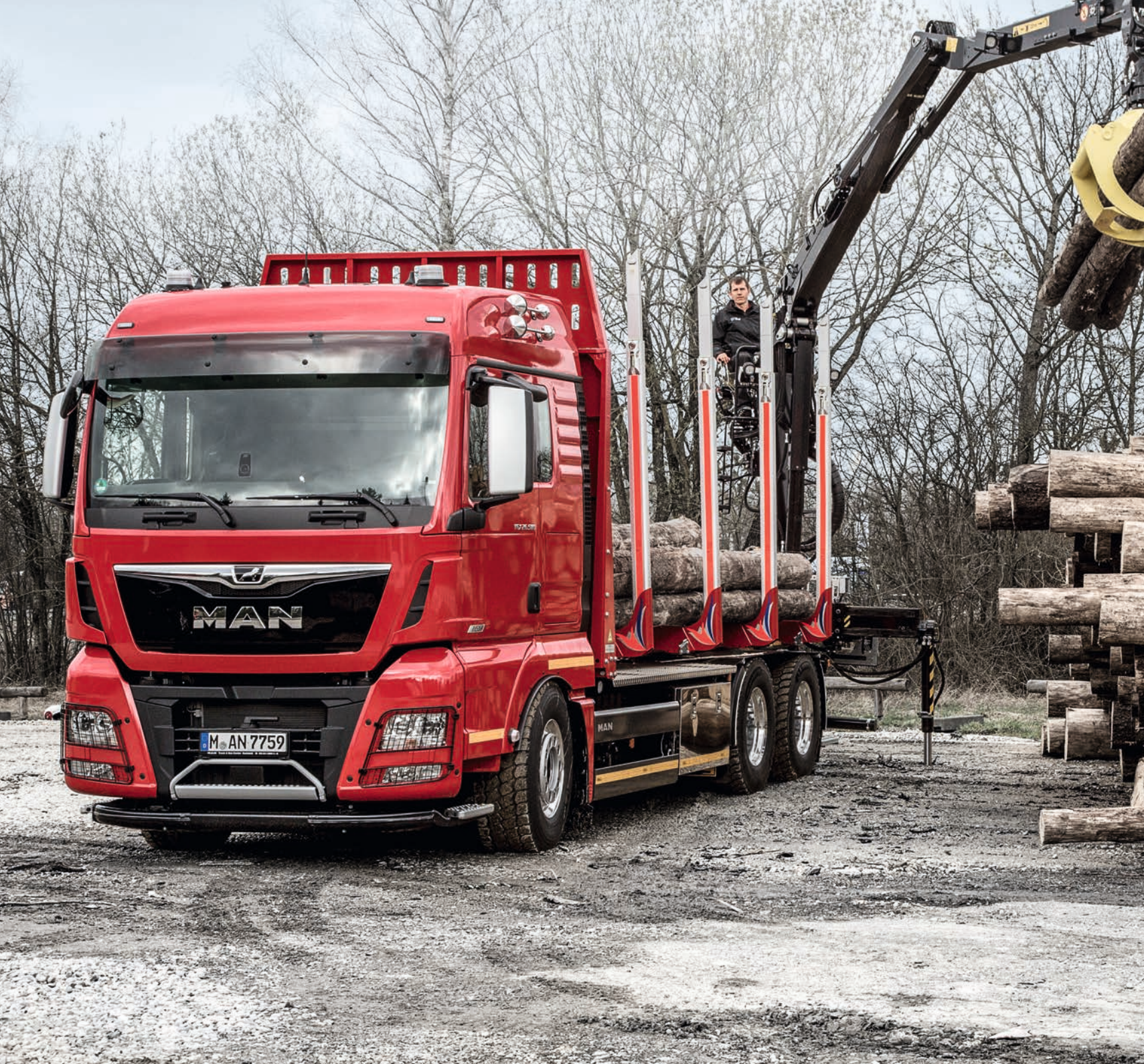
Steel bumper with robust protective grill for radiator and headlights
