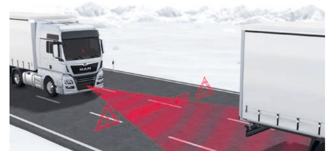
Functional principle EBA: advanced traffic monitoring by using two independent sensor systems (radar and video)
