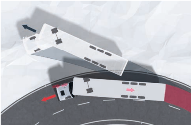
ESP compensatory braking when vehicle is oversteered.
