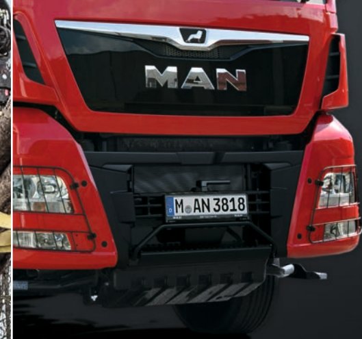
Steel bumper with robust protective grill for radiator and headlights
