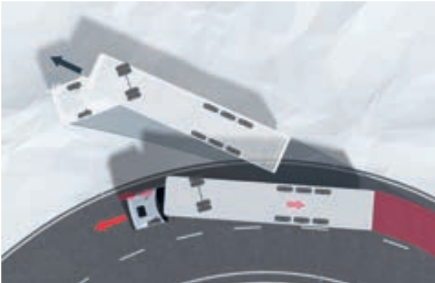
ESP compensatory braking when vehicle is oversteered.
