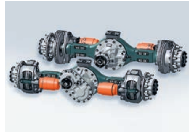
Light MAN TGS tandem hypoid axle
