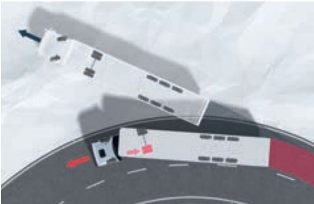
ESP compensatory braking when vehicle is understeered.
