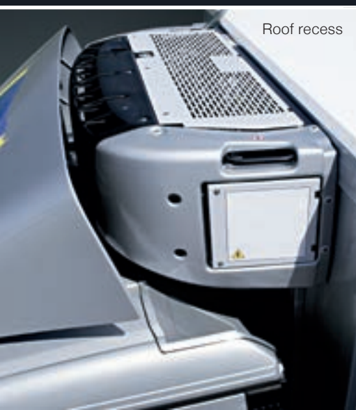
Fitting situation for Frigoblock generator
