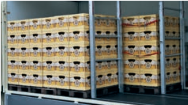
Example: securing of loads on body complying with VDI 2700
