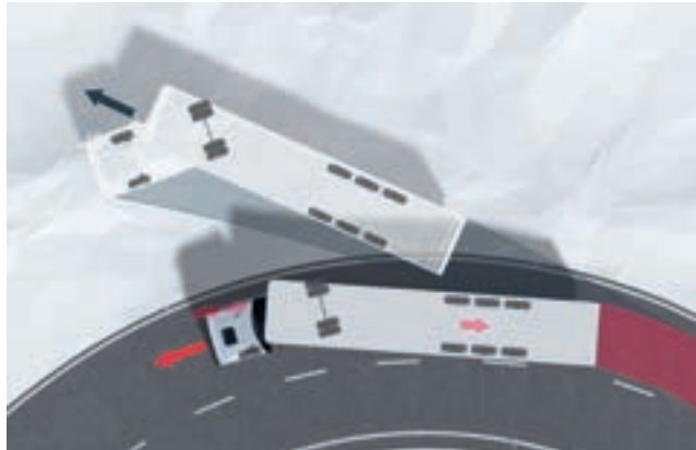
ESP compensatory braking when vehicle is oversteered
