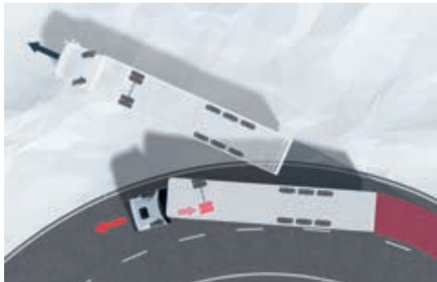
ESP compensatory braking when vehicle is understeered.
