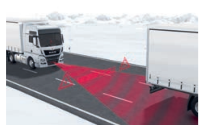
Functional principle EBA: advanced traffic monitoring by using two independent sensor systems (radar and video)
